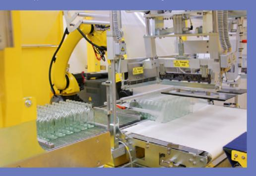
The second-generation of machine utilises servo controls and this latest edition now incorporates an integrated robot allowing easier size change, gentler bottle control and flexibility.
